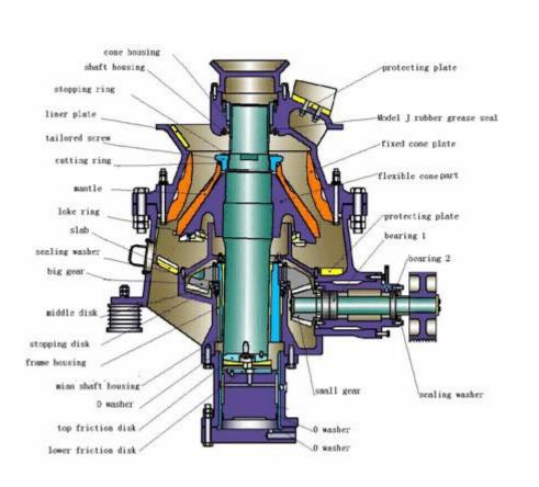
The motor drives the eccentric shaft bushing through V-belt, transmission shaft, and transmission gear. The cone makes circle movement at the force of eccentric shaft bushing, and close to mantle from time to time. Raw materials are crushed during the process and are later discharged at the bottom.
