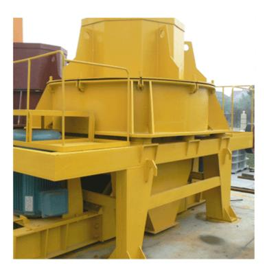
Therefore some materials will be impacted, crusher, milled twice or more times in the whirlpool cavity, then crushed materials will be excluded through the bottom discharginghole. This can from a closed circulation through the circular classifier system; in general, materials can be crushed into 20 mesh through thrice circulation. Airflow self-circulation in the whirlpool cavity can eliminate the dust pollution well.
